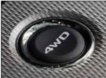
The drive mode can be switched by pressing the 4WD button while the ignition switch is in the ON position.
