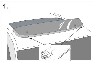
Open the sunroof and clean installation areas thoroughly. Trial fit Sunroof Deflector centrally on roof. Take note and mark the areas on Sunroof Deflector where rubber extrusion and metal clips are to be positioned. Remove Sunroof Deflector.
