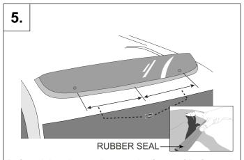
Before tightening, make sure the Sunroof Deflector is centered on the roof and that the clips are seated correctly and over the abrasive resistant tape. Ensure rubber seal is spread out flat against the roof and does not curl under at any point.
