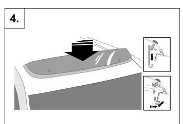
Re-fit the Sunroof Deflector centrally on the roof. Position clips at front of the sunroof opening. Depress the corners of the Sunroof Deflector to hook the clips under the inside edge of the opening.
