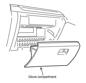
1) Remove the glove compartment in accordance with the workshop manual.
