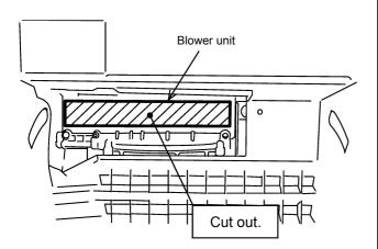
2) Confirm that this is the first time to install or replace the air filter. Check whether an air filter is already installed at the hatched section shown in the drawing (with two tapping screws).
