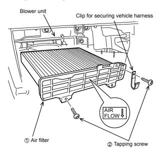
1) Install the air filter ① in the correct direction. The "AIR FLOW" arrow mark on the air filter should be pointing downward.
