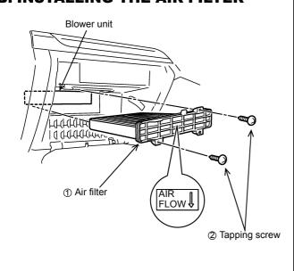
1) Install the air filter ① in the correct direction. The "AIR FLOW" arrow mark on the air filter should be pointing downward.
