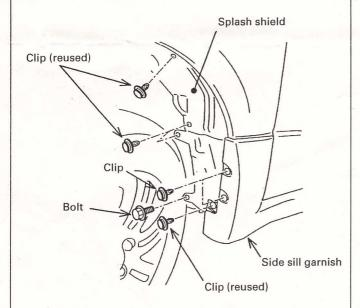
1) Remove six fixing clips and one bolt from the splash shield inside the front wheel well.
