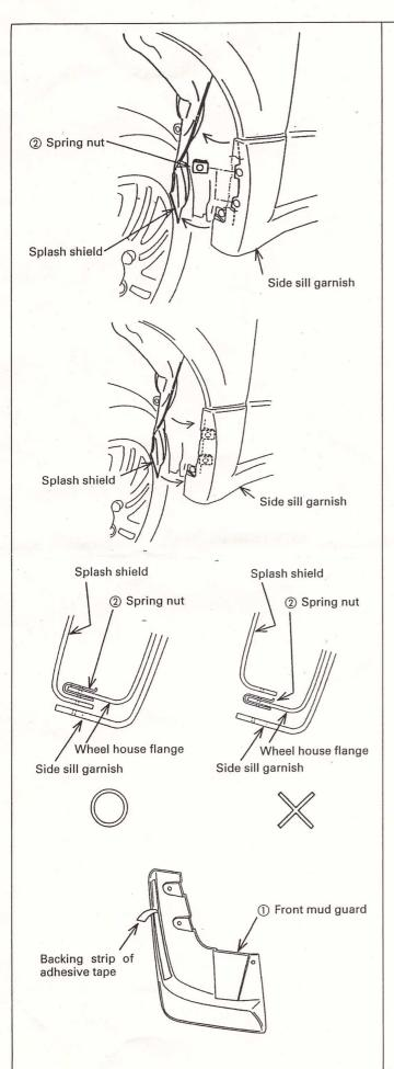
Pull open the splash shield and fit two spring nuts (2) onto the edge of the wheel house flange behind the side sill garnish, with their holes in alignment with the existing holes in the wheel house.
