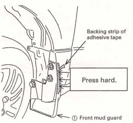
6) Restore existing splash shield clips in their original positions, then install the front mud guard ① as shown.
