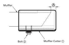
2) Position the Muffler Cutter ① as shown in the drawing.
