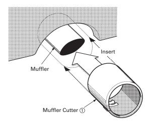
1) Place the Muffler Cutter (1) over the muffler.
