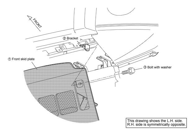
3) Temporarily install the rear of the front skid plate ① to the existing front skid plate mounting holes with removed bolts.
