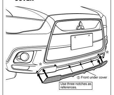
1) Place the front under cover ① on the front bumper to confirm its mounting position. Using the three notches at the top of the front under cover ① as references, position the under cover ① so that the left and right gaps at the positions marked with ☆ in the drawing become equal.
