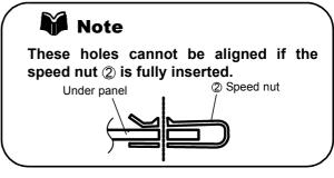
3) Reinstall the front bumper while taking care not to move the aligned speed nuts ②. When reinstalling, however, do not attach the seven clips at the positions shown in the drawing in **B**-6).
