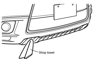
Clean and degrease the under cover ① mounting position on the front bumper using clean shop towel moistened with isopropyl alcohol or degreaser.
