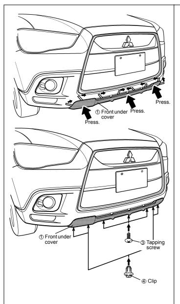
5) Peel off the remaining backing strips slowly and carefully and then press the under cover ① against the bumper firmly.
