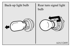
6. To install the bulb, perform the removal steps in reverse.
