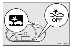
If the indicators remain even after the ignition switch is turned to the "OFF" position and then turned back to the "ON" position or the operation mode is put in OFF and then turned back to ON, please contact your authorized Mitsubishi Motors dealer.
