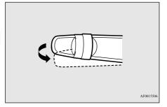
4. The headlights will come on in the low beam setting for approximately 30 seconds. After the headlights go off, the headlights can be turned on again in the low beam setting for approximately 30 seconds by pulling the turn signal lever toward you within 60 seconds of turning the ignition switch to the "OFF" position or putting the operation mode in OFF.
