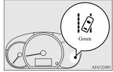
To turn off the LDW, press the LDW switch. The LDW indicator (green) in the meter cluster will then go out.
