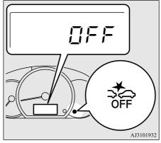
To turn on the FCM again, press and hold the FCM ON/OFF switch. The indicator on the instrument cluster will go off, and a current distance mode for the forward collision warning will be shown in the multi-information display.
