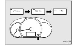
2. Press and hold the multi-information display switch for about 1 second or more to make the wrench symbol start flashing. (If there is no operation for about 10 seconds with flashing, the display will revert to its original indication.)
