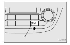
After about 20 minutes of operation, the system will shut off automatically.
