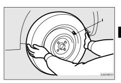
7. Install the wheel nuts with their tapered ends facing inward, then tighten by hand until the wheel is no longer loose.
