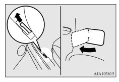
Open the fuel tank filler pipe by slowly turning the fuel tank filler cap counterclockwise.
