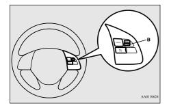
To slow down your speed in small amounts, press the SET - switch for less than about 1 second and release it.
