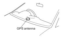
The location of your car is measured by receiving weak radio signals from GPS satellites with the "GPS antenna"
