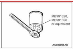
Use the respective tool in the following table to remove the engine oil filter.
