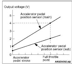
The relationship between accelerator opening angle and output voltage of the accelerator pedal position sensor (main) and accelerator pedal position sensor (sub) is as shown in the figure.
