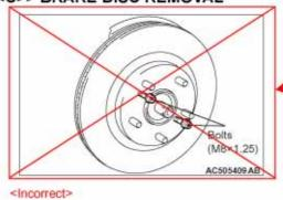
If the brake disc removal is difficult, install bolts (M8 x 1.25 mm) shown in the figure, and tighten them evenly and gradually to remove the brake disc.
