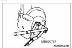
Use special tool front hub and flange yoke holder (MB990767) to counter the hub as shown in the figure to remove the driveshaft nut.
