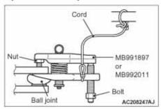
Install special too ball joint remover (MB991897 or MB992011) as shown in the figure.
