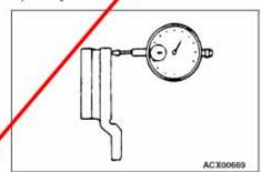
Set a dial gauge on the brake disc approximately 5 mm inside the periphery, and measure the runout of the brake disc.
