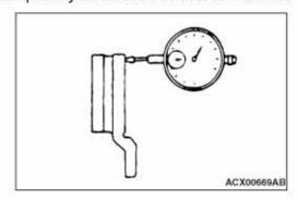
Place a dial gauge approximately 5 mm from the outer circumference of the brake disc, and measure the run-out of the disc.
