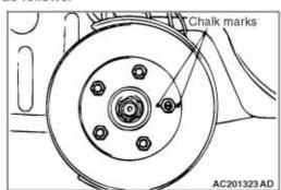
Chalk phase marks on the wheel stud and the brake disc, which run-out is excessive as shown.
