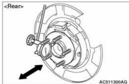
(2) Remove the brake disc. Set a dial gauge as shown in the figure, and measure looseness of the hub in the axial direction.
