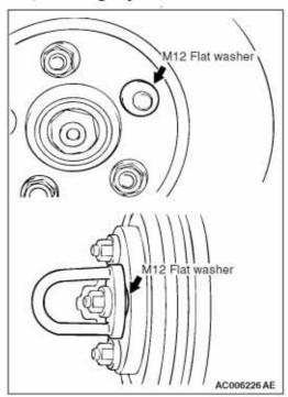
When the on-the-car type lathe is used, first install M12 flat washer on the stud bolt in the brake disc side according to the figure, and then install the adapter. If the adapter is installed with M12 flat washer not seated, the brake disc rotor may be deformed, resulting in inaccurate grinding.
