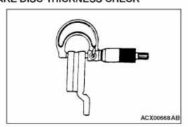
Using a micrometer, measure disc thickness at eight positions, approximately 45 degrees apart and 10 mm in from the outer edge of the disc.
