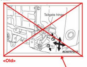
If the clearance between the tailgate and the vehicle body is uneven, remove the rear bumper assembly (refer to GROUP 51 - Rear Bumper) and loosen the body-side tallgate hinge mounting nuts to adjust the tailgate lower so that the clearance between the tailgate and body becomes even.
