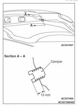
Rotate the damper by using the arrow mark on the damper as a guide to adjust the tailgate height. The damper height is altered by roughly 3 mm when the damper is rotated once.
