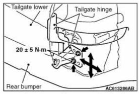
Loosen the tailgate hinge mounting bolts as shown in the illustration located at left and right sides of the body, and slide the tailgate lower to adjust its position so that the clearances between the tailgate lower and body (rear bumper assembly) at left and right become even.
