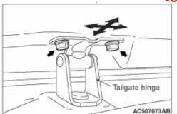
If the clearance between the tailgate and the body is uneven, loosen the tailgate-side tailgate hinge mounting bolts to adjust it.
