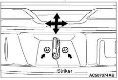
If the striker is not engaged with the latch properly, adjust by loosening the striker mounting screws.
