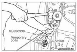
If the striker is not engaged with the latch properly, remove the quarter trim lower (Refer to GROUP 52A - Interior Trim ). Replace the striker mounting screw with an adequate bolt, and use special tool remover bar (MB990939) and a hammer to tap the bolt head in the desired direction to adjust the striker.
