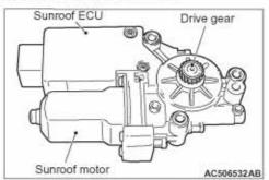
The sunroof motor assembly, which consists of the motor main body, drive gear, and sunroof ECU, is installed in front of the housing.
