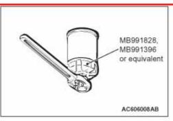
Use the respective tool in the following table to remove the engine oil filter.
