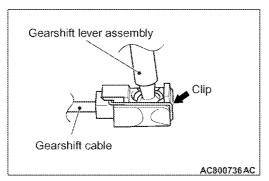
When removing the gearshift cable, be careful not to deform it because the clip is opened forcibly.
