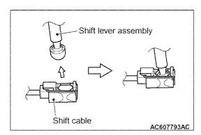
After the installation, slightly pull the joint to down direction to check that it is connected securely.
