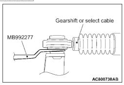
Be careful not to pull out the cable directly to disconnect the joint because the cable could be broken.
