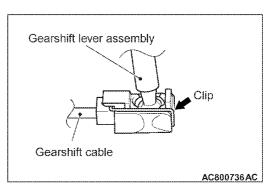
When removing the gearshift cable, be careful not to deform it because the clip is opened forcibly.
