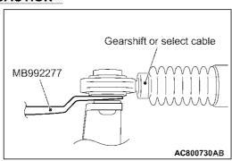
Be careful not to pull out the cable directly to disconnect the joint because the cable could be broken.
