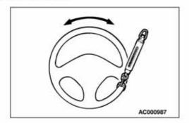
Measure the circumferential steering wheel play until the front wheels actually start operating while turning the steering wheel slightly in the left and right directions.
