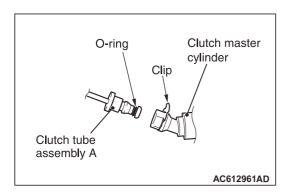
CLUTCH TUBE ASSEMBLY A CONNECTION < Added>
