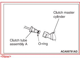
**CLUTCH TUBE ASSEMBLY INSTALLATION**
