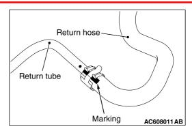
4. Align the making as shown in the figure and connect return hose. Then install the steering gear and linkage. <LHD>
