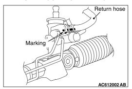
Install the return hose by aligning the mating marks. <a href="RHD">RHD</a> <a href="Added">Added</a>
