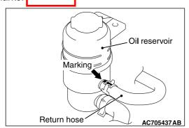
2. Install the return hose with its marking located as shown in the figure.
