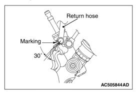
1. Align the marking as shown in the figure and connect the return hose. <a href="#">RHD except 3000></a>
