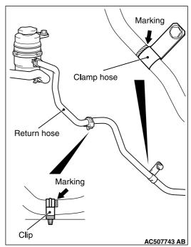
3. Using clip and hose clamp align the return hose marking within the area shown in the figure and connect the return hose<2400>.
