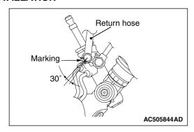
1. Align the marking as shown in the figure and connect the return hose. <RHD> <Added>
