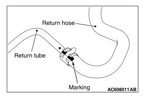
Align the making as shown in the figure and connect return hose. <LHD>
