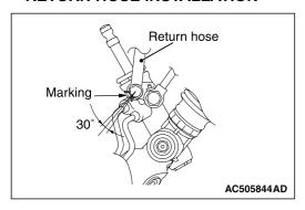
Align the marking as shown in the figure and connect the return hose.
