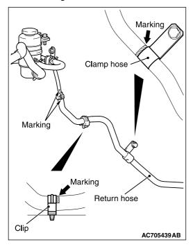
3. Using clip and hose clamp, install the return hose with its marking located as shown in the figure.
