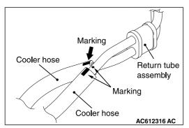
Align the marking as shown in the figure and connect the cooler tube hose.
