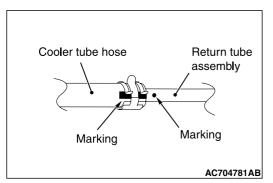
Align the making as shown in the figure and connect cooler tube hose.
