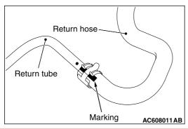
Align the making as shown in the figure and connect return hose.
