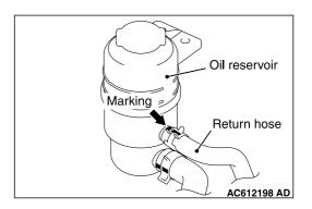
2. Align the return hose marking within the area shown in the figure and connect the return hose.
