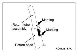
3. Align the making as shown in the figure and connect return hose.
