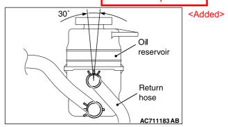
2. Align the marking within the area shown in the figure and connect the return hose.
