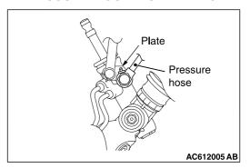
Install the pressure hose plate with its marking located as shown in the figure.
