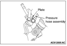
Align the pressure hose plate as shown in the figure and connect pressure hose assembly.
