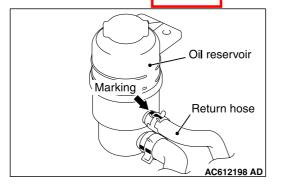
Using clip and hose clamp align the return hose marking within the area shown in the figure and connect the return hose.
