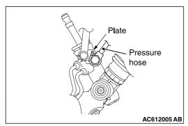
Align the pressure hose plate as shown in the figure and connect pressure hose.
