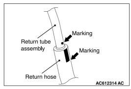
Align the marking as shown in the figure and connect the return hose.
