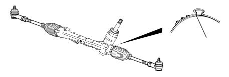
· Special tool:MB992908(Bellows band clipping tool)
