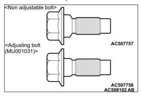
(3) If adjustment is not possible, replace the doorside door hinge mounting bolt with the adjustment bolt (MU001031).
