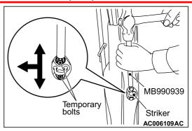
(1) Adjustment using the striker (toward the inside of the vehicle and vertical direction): Install a temporary bolt instead of the striker mounting bolt, and use the remover bar (Special tool: MB990939) and a hammer to tap the temporary bolt to the desired direction.
